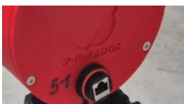
Ethernet cable connection to the case
